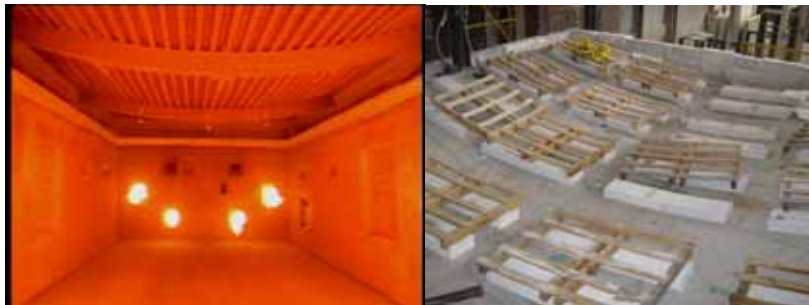
Figure 7.38 Tested floor during and after the fire
