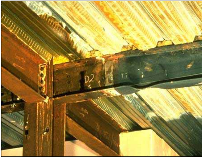
Figure 2.5 Flange buckling in restrained beam
